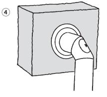
Finish with the flue rosette to seal the installation.
