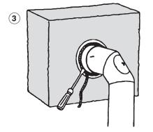
Stuff with tow material between the flue and the wall mounting connectors.
