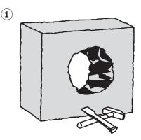
Carefully make a hole in the spot where you will connect your stove to the chimney stack.
